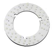
**Overview :** Replacement Board with 90 LEDs for 26501-LED
