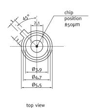
UVB-only SiC based UV photodiode A = 0,06 mm<sup>2</sup>
