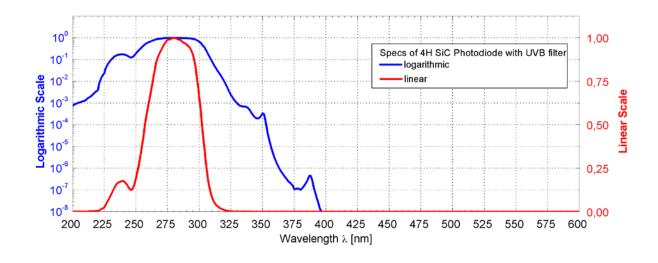
UVB-only SiC based UV photodiode A = 0,06 mm<sup>2</sup>
