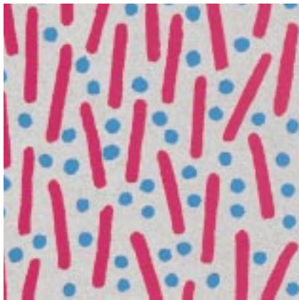
Illustration 200.6: The structure of iglidur® : base polymer, fillers and solid lubricants
