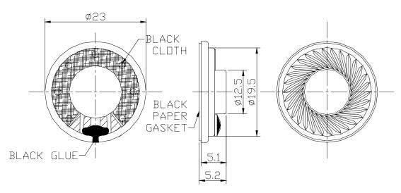
Dimensions : Millimetres Tolerance: ±0.5mm
