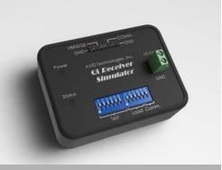
The Qi FOD Receiver is a power receiver that can be placed on Qi wireless transmitters and used to test the operation and FOD performance. DIP switches on top of the FOD Receiver are used to program received power offsets and to change internal loads.
