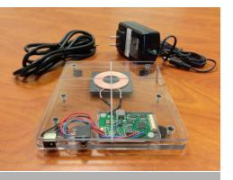
The Qi FOD Transmitter is a V1.1 power transmitter that can be used to test the operation and performance of Qi V1.1 power receiver devices. A USB serial interface is used to display operating information and to program transmitted power offsets as well as change the operating modes.
