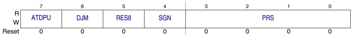
Figure 14-3. ATD Control Register (ATDC)
