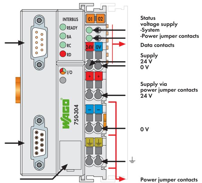
This buscoupler connects the WAGO-I/O-SYSTEM as a slave to the INTERBUS fieldbus.
