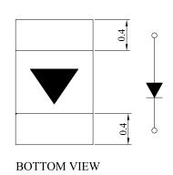
All dimensions are in mm Tolerance: ±0.1mm
