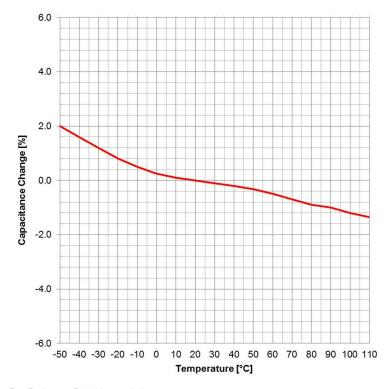
Test Equipment: E4991A or equivalent
