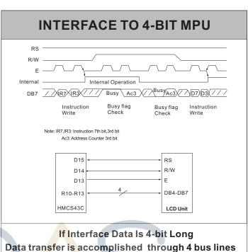
from DB4 to DB7. (while the rest of 4 bus lines from
