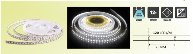
This daylight LED strip has 120 LEDs per metre and is constructed using high quality materials to ensure a consistent light and colour across the strip. This LED strip is IP33 rated and is suitable for indoor applications. Each 5m reel is supplied with an easy-to-follow installation guide and an extra connector (Connector end to strip and 15cm wire to power) to power the strip if it is cut into two lengths. 3M backing tape is pre-applied to simplify the installation process.
