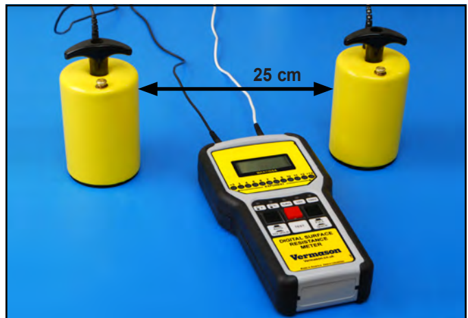
Figure 6. Rp-p test setup - set the electrodes about 25 cm apart for working surfaces and about 1 m apart for flooring
