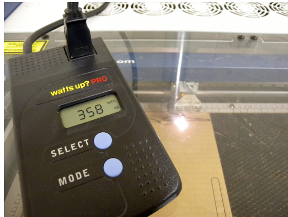
Figure 1-3. Digital watt meters can accurately display a piece of equipments' power consumption in real time.
