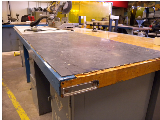
Figure 1-8. Covering work surfaces with inexpensive and durable materials helps to prolong the life and quality of the work surface.
