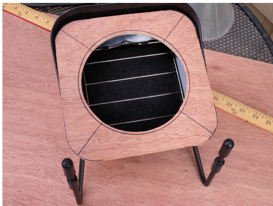
Figure 1-14. Use a coping saw or jig saw to cut out the large hole in the center and outline of the plywood plate.
