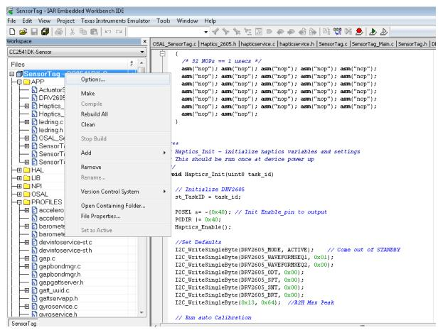
5. Navigate to Linker and under the linker configuration file, select *Override default* and select the "ti\_51ew\_cc2540b.xcl" file from the previously unzipped cc4540 folder.
