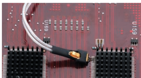
N5439A InfiniiMax III ZIF probe head soldered in to an IC
