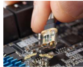
N2848A QuickTip head with N2849A QuickTip tips
