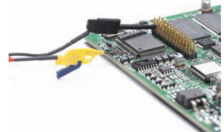
IC clips included in N2877A and N2878A accessory kits for N2870A Series passive probes
