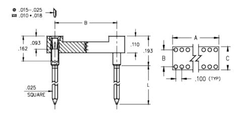
**Description:** DIP Dual In Line Socket Wire-Wrap Tail Open Frame **Plating Code:** Shell Plating:  $10~\mu"$  Gold over 100  $\mu"$  Nickel
