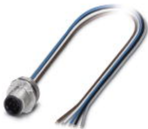
Fieldbus flush-type plug, INTERBUS/PROFIBUS, 5-pos., M12 SPEEDCON, B-coded, front/screw mounting with M16 thread, with 0.5 m TPE litz wire, 5x0.25 mm 2
