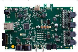
The xCORE-200 Multichannel Audio Platform provides a scalable and flexible hardware and software solution for a wide range of consumer and professional audio products.
