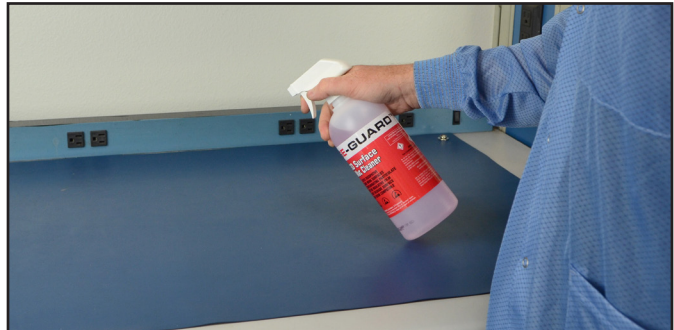
Figure 2. Applying Charge-Guard™ to the mat.
