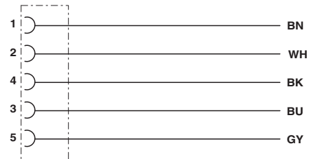
Contact assignment of the M12 socket
