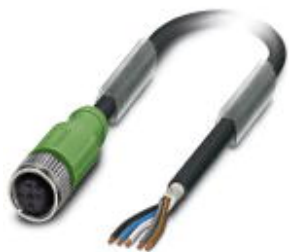
Sensor/Actuator cable, 5-position, PUR halogen-free, black-gray RAL 7021, shielded, free cable end, on Socket straight M12, A-coded, Cable length: 3 m
