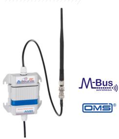
The combination of products in the **Adeunis RF AMR range** allows you to **create an independent ecosystem** to ensure the emission, transport and collection of consumption indexes using Wireless M-Bus protocol.
