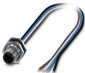
Bus system flat-type plug, 4-position, PlugLink:M12, D-coded, Rear mounting, M16 x 1.5, Individual wires, Cable length: 0.5 m
