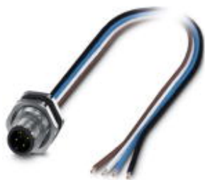
Flush-type connector, Universal, 5-position, PlugLink:M12, A-coded, Rear mounting, M16 x 1.5, Individual wires, Cable length: 0.5 m
