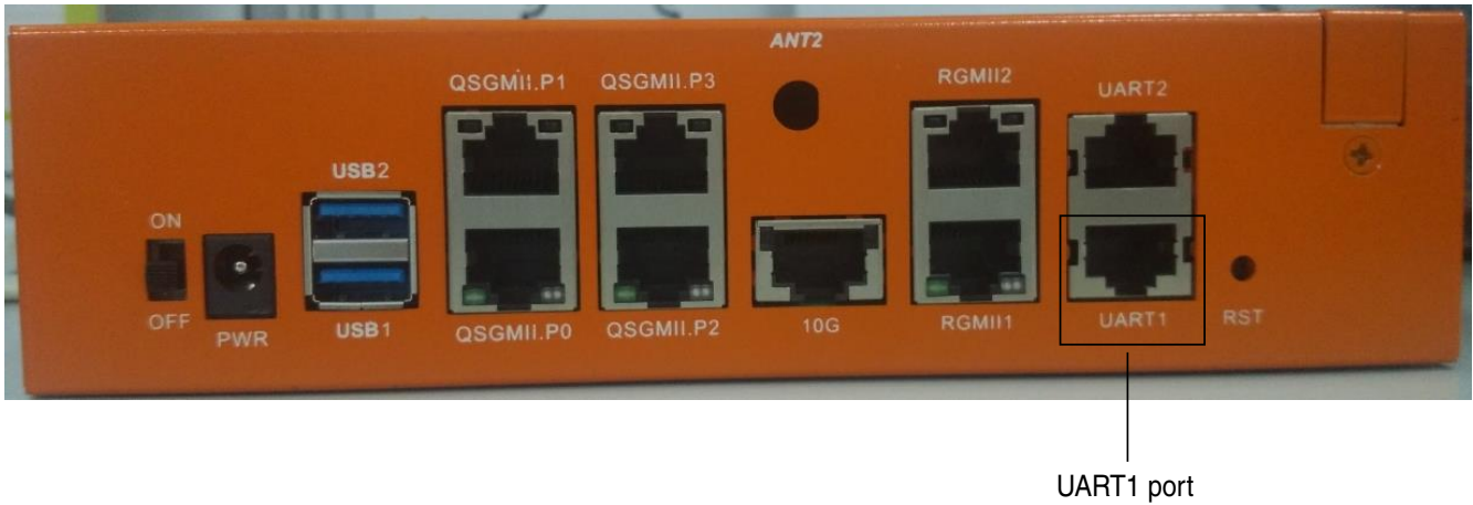
Figure 8. UART1 connection using RJ45 connector
