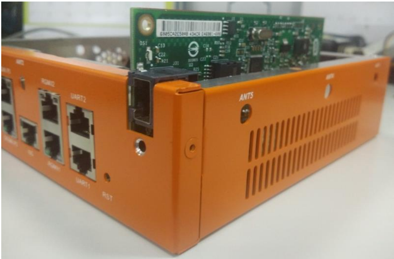
Figure 11. Standard PCI express card installation
