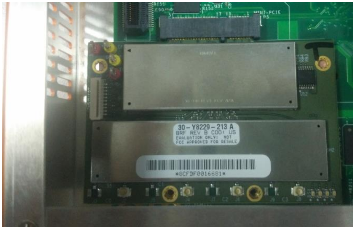
Figure 13. Mini-PCI express card installation
