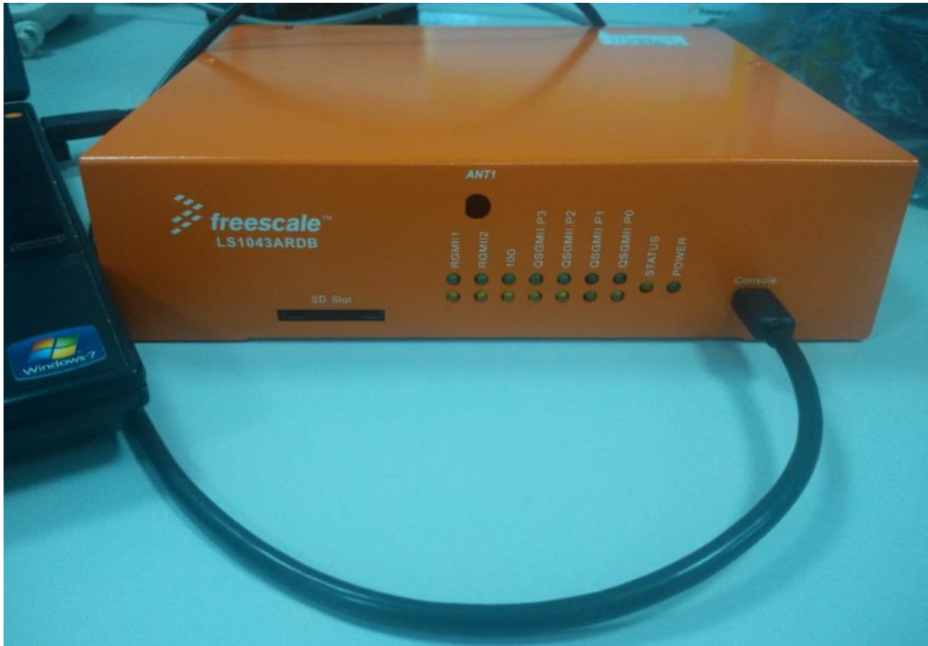
Figure 9. UART1 connection using mini-USB
