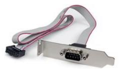
The PLATE9M16LP (16 inch/ 0.4 m) Low Profile Serial Plate adds a DB9 serial port to the rear panel of a small form factor/low profile computer, connecting to an IDC10 header connector on the motherboard.
