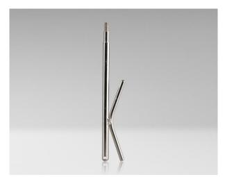
K hook specially designed for push and pull cable installation and retrieval operations. K hook cable to handle cables up to 3/8" diameter. Has standard 8-32 thread for use on fish sticks and glow rods.
