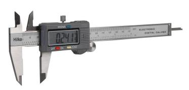
Durable stainless steel construction in plastic case. Zero calibration switch with automatic on/off easy to read LCD screen. Suitable for taking internal, external and depth measurements with maximum measuring range 150mm (6").
