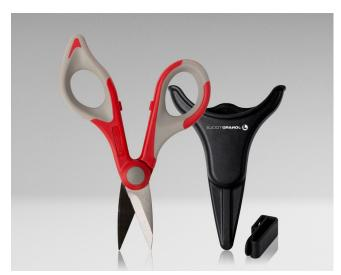
JIC-186 Ergonomic Fiber Optic Kevlar Cutter in a molded pouch with belt clip. High carbon stainless steel blades designed to cut Kevlar®, cabling insulation, tape, cable ties and other material. Ergonomic handles for user comfort and durability. Adjustable joint screw under protective cap, serrated blades grip material, sharp and durable 6" long
