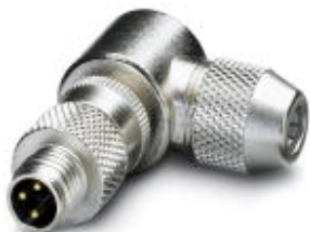
Connector, 3-position, shielded, Plug angled M8, A-coded, Solder connection, Knurl material: Nickel-plated brass, External cable diameter 3.5 mm ... 5 mm
