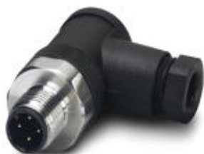
Sensor/actuator connector, male, angled, 4-pos., M12, screw connection, high-grade steel knurl, cable screw connection Pg7
