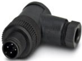
Connector, 4-position, Plug angled M12, A-coded, Screw connection, Knurl material: Plastic, Cable gland Pg7, External cable diameter 4 mm ... 6 mm
