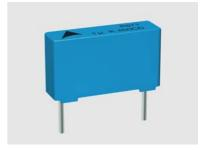
The new series comprises types with lead spacings of 10 mm, 15 mm and 22.5 mm, respectively. The capacitors are designed for rated voltages of 450 V DC, 520 V DC and 630 V DC and cover a capacitance range from 68 nF to 2.2 µF. These components are suitable for a continuous operating temperature of 125 °C. The plastic of the case satisfies UL 94 V-0 specifications. Halogen-free versions are also available upon request.
