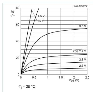
Output characteristics; drain current as a Fig. 7. function of drain-source voltage; typical values
