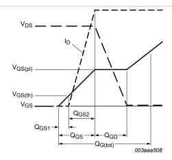
Fig. 13. Gate charge waveform definitions
