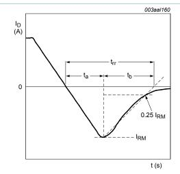
Fig. 16. Reverse recovery timing definition
