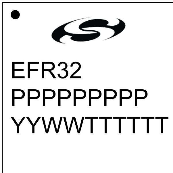
Figure 8.3. QFN32 Package Marking
