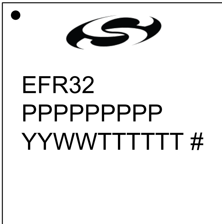
Figure 7.3. QFN48 Package Marking
