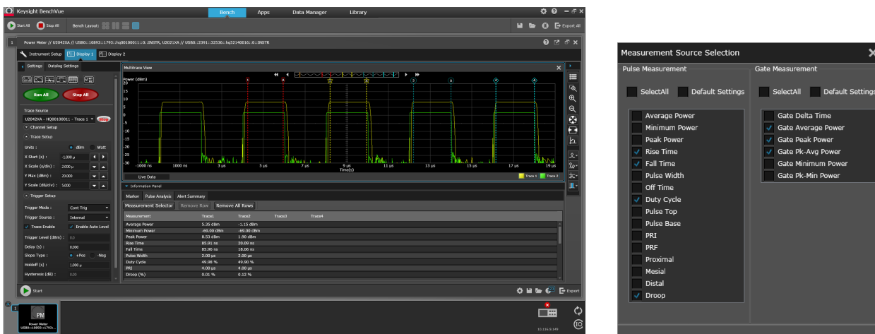
Figure 9. Multi-channel trace display with 4-pairs of gates and automatic pulse parameters measurement (sample screen shot with U2021XA and U2042XA)
