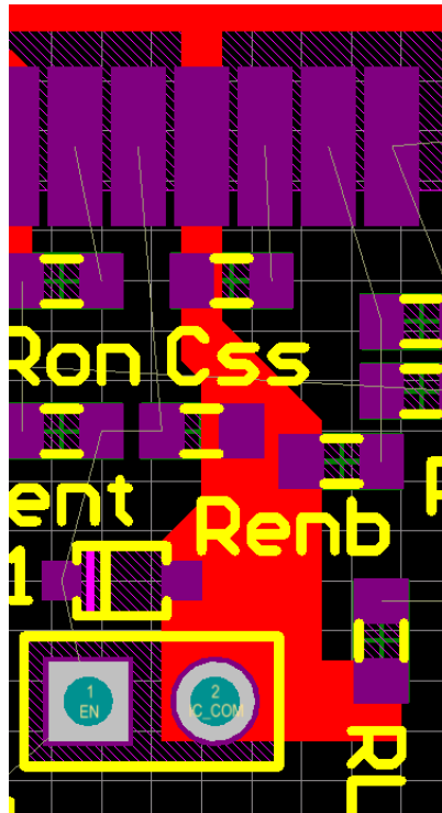
Figure 21: Single-point connection of all the analog components to the AGND pin and then to the power pad
