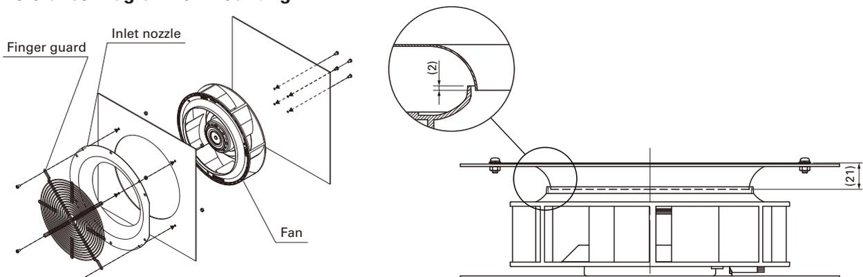
The screw length is 6 mm less or equal from fan edge side.
