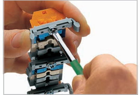
Terminal strip with fixing flanges, screw mounting of 209-123 mounting adapter (The distance between mounting adapters should be 25 - 30 mm).
