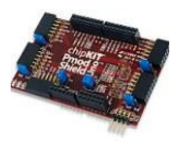
The chipKIT<sup>TM</sup> Pmod Shield is an input/output expansion board for use with the chipKIT uC32 (TDGL017) or chipKIT Uno32 (now discontinued), as it has the same form factor. With five 2x6 Digilent Pmod connectors, access to available I/O connectors on the base boards, and connectivity to the supported I2C bus, this Pmod Shield provides all the additional circuitry and connections to allow Digilent Pmods to be used with these two chipKIT base boards.
