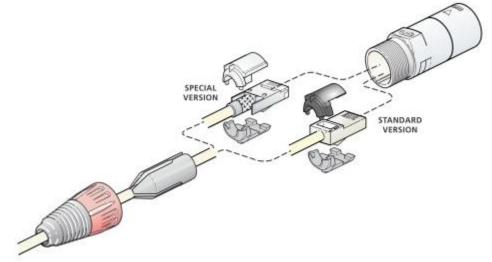
By help of the new alignment system we now support a greater range of RJ45 plugs while in parallel the improved positioning grants a smooth mating with the corresponding etherCON receptacle. Additionally, we significantly eased the assembly of the connector since the chuck now clasps around both alignment parts and so it is very convenient to insert the assembly group into the housing.
