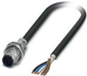
Flush-type plug, shielded, 5-pos., M12, A-coded, rear/screw mounting with M16 thread, with 1 m cable, 5 x 0.34 mm 2
