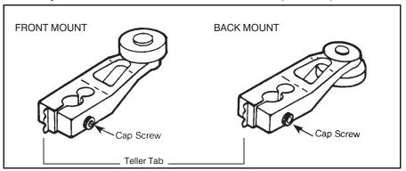
Levers shown in the order guides are furnished with cap screws which accommodate a %4-inch allen wrench.
