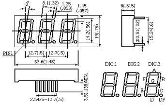
Dimensions : Millimetres Tolerance : ±0.25mm
