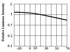
$\label{eq:ambient Temperature Ta= $^{\circ}$C} \\ Luminous Intensity vs. Ambient Temperature$
