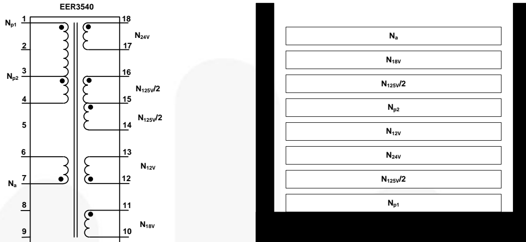
Figure 42. Transformer Schematic Diagram
