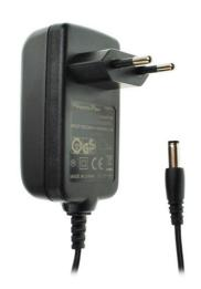
This switch mode power supply is rated to 12W maximum, providing a regulated 24vdc output at up to 0.5A with no minimum load. The unit meets Level VI COC Tier 1 efficiency standards. This power supply carries full safety approvals. Short circuit and over current protection is integral.
