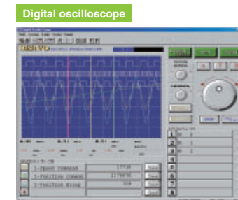
●Collect and confirm the motion system's time-series operation state without using a real oscilloscope.
