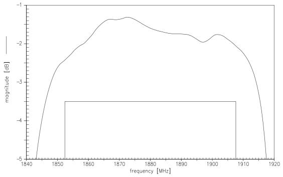
Transfer function for WCDMA signals (Powertransferfunction vs. carrier frequency)
