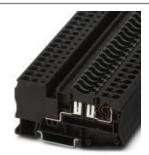
Fuse modular terminal block, Connection method: Spring-cage connection, Cross section: 0.08 mm²- 6 mm², AWG: 28 - 10, Nominal current: 30 A, Nominal voltage: 400 V, Width: 8.2 mm, Fuse type: C, Fuse type: Flat, Mounting type: NS 35/7,5, NS 35/15, Color: black
