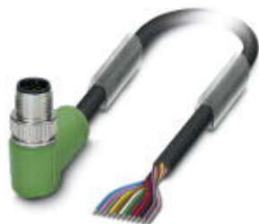
Sensor/Actuator cable, 12-position, PUR halogen-free, black RAL 9005, Plug angled M12 SPEEDCON, A-coded, on free cable end, Cable length: 3 m
