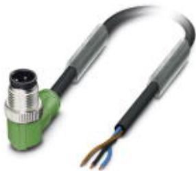
Sensor/Actuator cable, 3-position, PUR halogen-free, black-gray RAL 7021, Plug angled M12, A-coded, on free cable end, Cable length: 3 m
